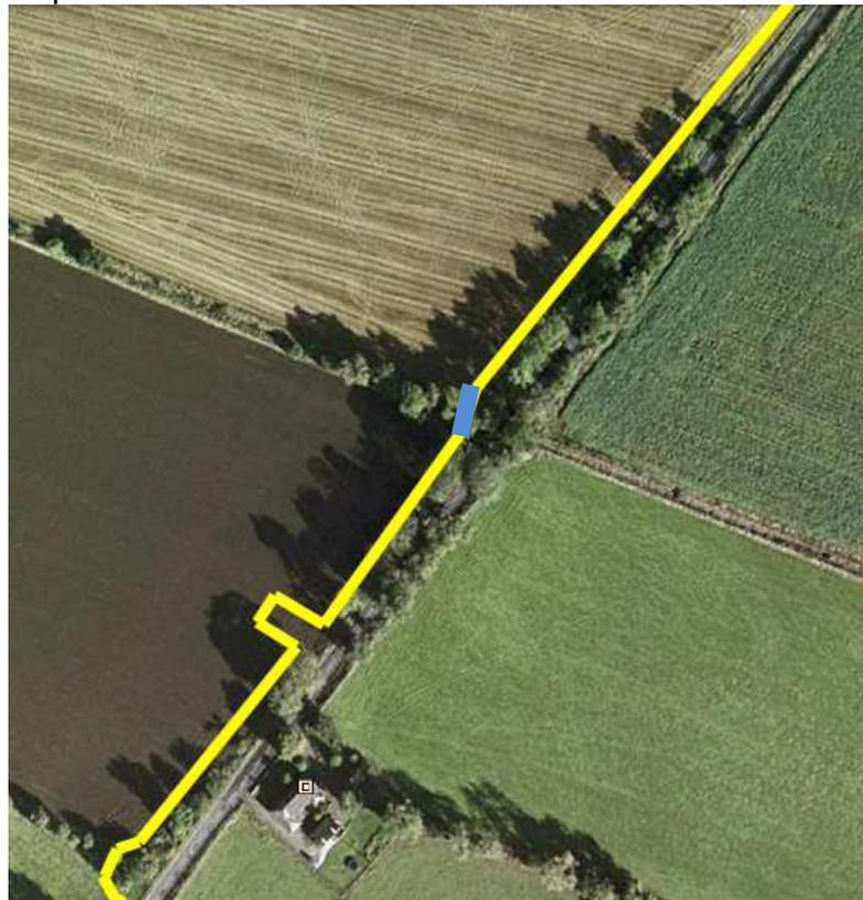
A burn will require a small bridge structure to be built here and again a 12m deviation can be seen.
