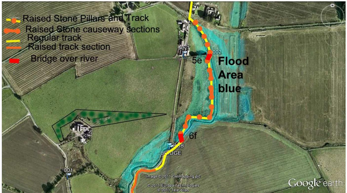
The above illustrates the extent of flooding. Depth of flooding in centre area adjoining Lochter Burn expected to be 1.3 m deep in parts every 2 years or so shown in blue. Proposed direct route of cycleway shown here will necessitate the building of a causeway as described below.
