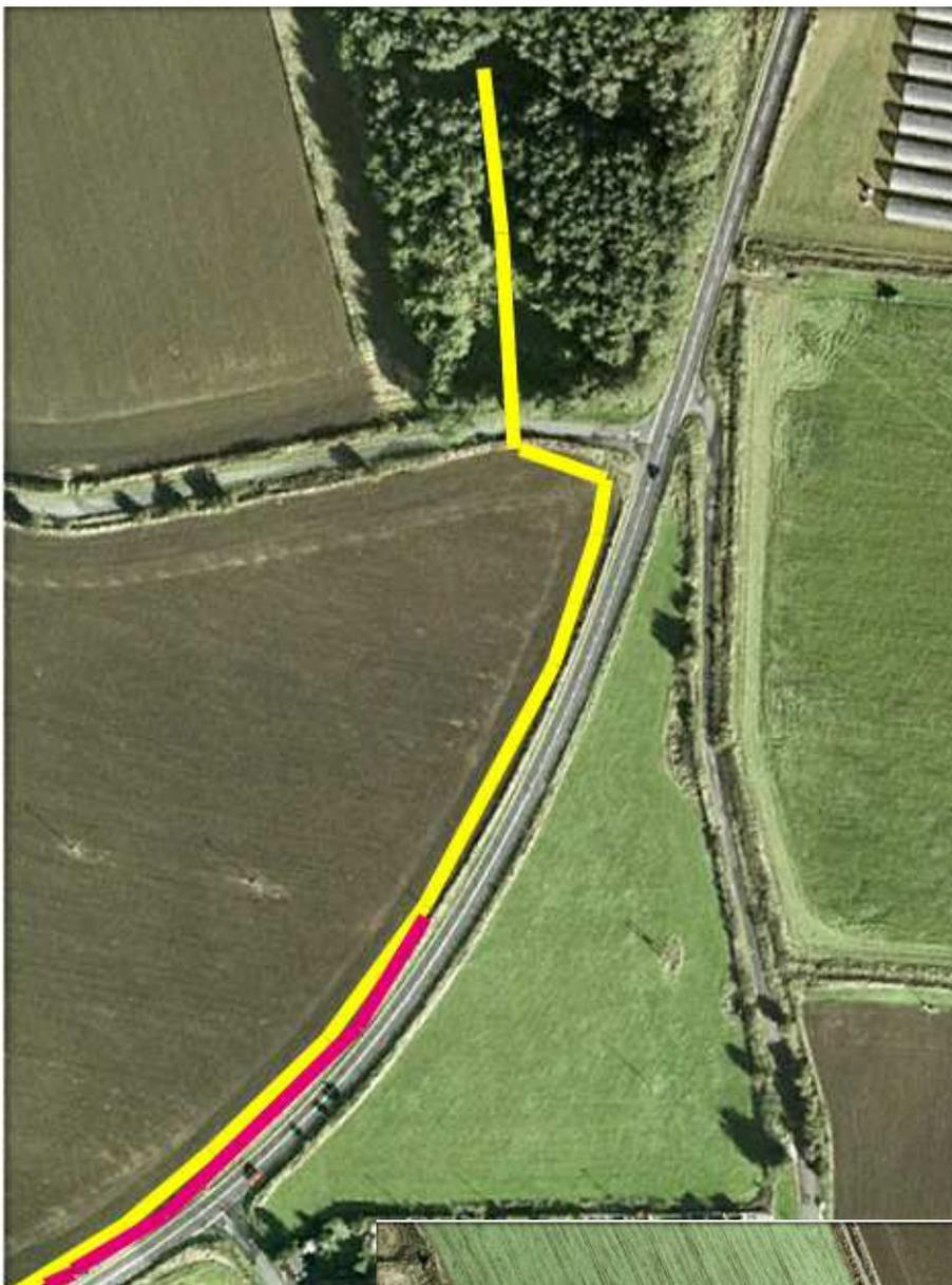
After the trees, the first road crossing near a junction requires the path crossing to be set well back from the junction as shown. Traffic has priority here. Cyclists and walkers give way.
