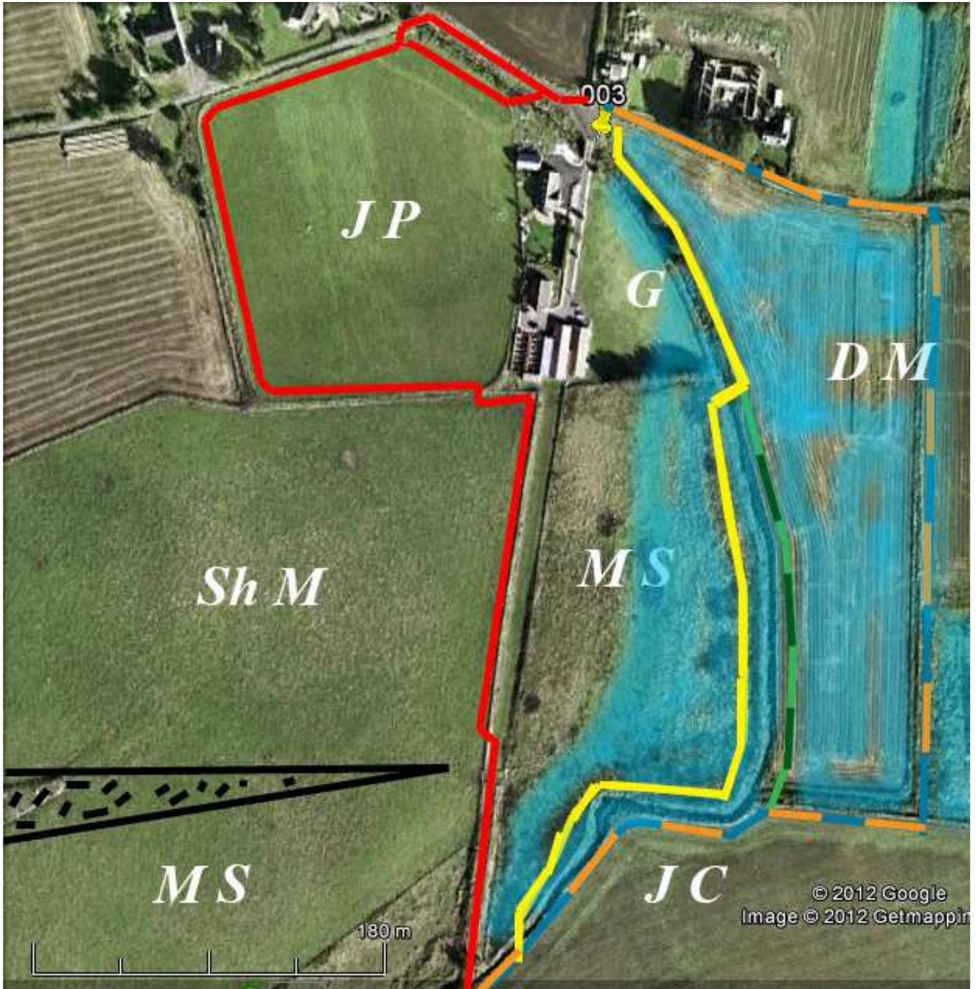
Alternative solutions come from re routing away from the flood plain. As badgers are not a problem, continuing along the original rail line over a new bridge ( $3.7 + 3.7 + 3.7 \text{ m} = 11.1\text{m}$  total span) along the red path might be possible if owner approval is forthcoming. i.e. Martin Sissons. His plans for a future hydro scheme using the bridge supports, may well be compatible.
